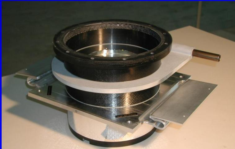
Non-metallic composite support post for magnets, with heat intercepts
