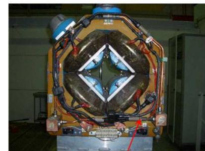
Brazed copper tubes with Vetronite insulators
