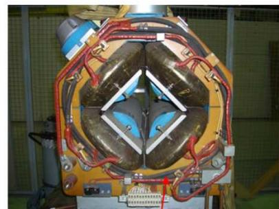
SPS injection line quadrupole Q1
