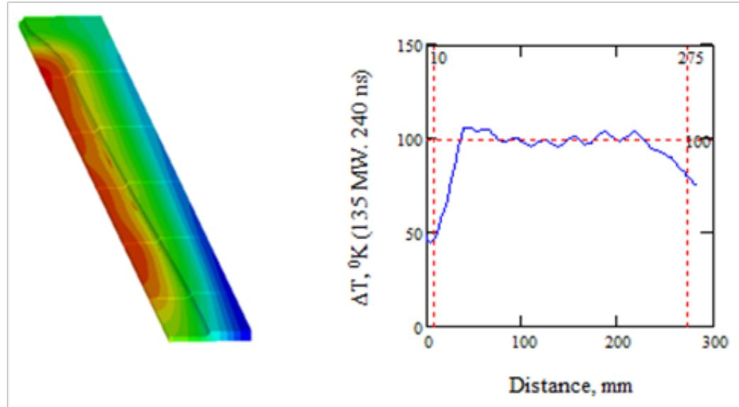
The magnetic field distribution on the quarter geometry of the single period tapered part is shown left. The pulsed heating profile along initial load length is shown right
