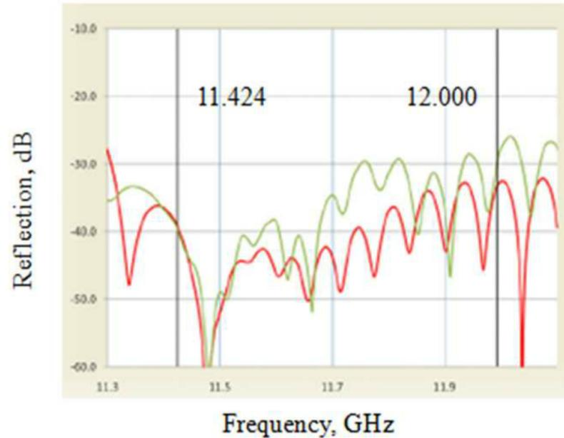
Measured (red) and calculated with HFSS (green) reflections in the typical load
