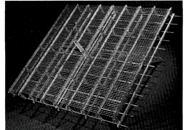
The microwave power transmission demonstration in 1975 at JPL Goldstone Facility. Distance between transmitting and receiving antenna was **1 mile**. Over **30kW** of DC power was obtained from the rectenna with a ratio of DC output to incident microwave power of **0.84**. Part of DC output was used to energize a bank of lights.
